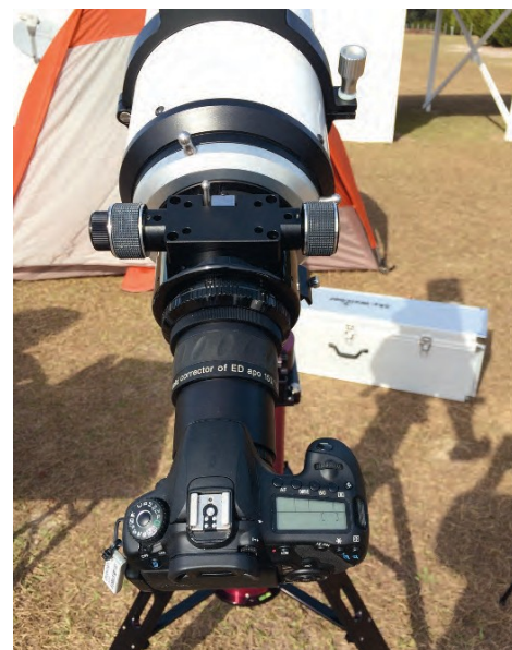
Image 4 - The Esprit 150's beefy focuser features a 1:10 fine-focus knob and an extra rail to prevent flexure under heavy loads. Shown also is the included field corrector securing a Canon 60Da.
